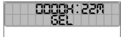
9. The third and last screen will display the battery charge status and the total run time of the machine. When the batteries are fully charged, the bottom line contains ten light indicators. As the batteries discharge, the indicator bars will go out and when the batteries are fully discharged the battery outline will begin flashing.
