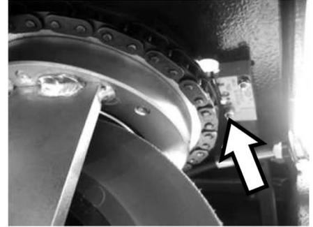
When the microswitch is activated, there should be 0.5 mm of clearance between the lever and the body of the switch. Check that the lever of the switch operates correctly.
