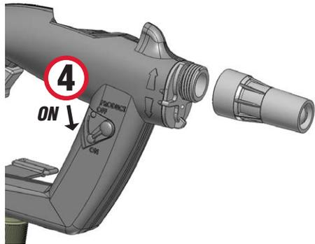
5. Depress trigger to begin dispensing desired concentrate solution; release trigger to stop flow of solution. To lock trigger in "ON" position depress and hold trigger while sliding red lock button back then release trigger. To release lock push red lock button up and slightly forward to stop flow of solution.
