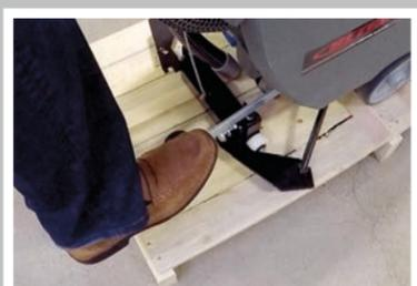
Press and lock pedal on rear right side of machine to lift scrub deck.
