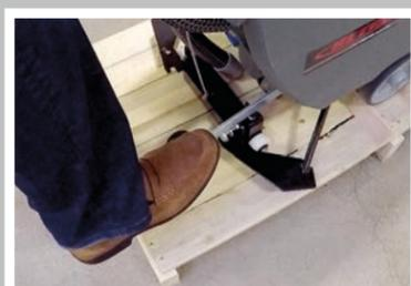
Lift scrub deck via pedal on rear right of machine.
