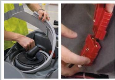
Locate and remove the splash guard from the recovery tank housing.
