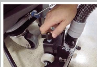
Adjust squeegee to desired height using guide wheel wing nuts.
