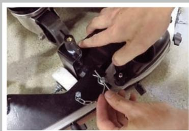
Install squeegee assembly by aligning at rear of machine and attaching retaining pins.
