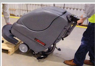
Carefully reverse the machine off the back of the pallet.
