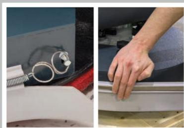
To install splash skirt, engage metal rings with connector nut, and wrap skirt around scrub deck. Lower scrub deck to the floor with your pad/brush installed and slide skirt down to contact the floor.
