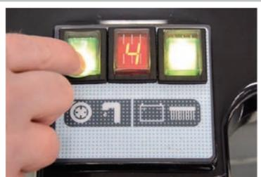
Press to activate brush and suction switch on the machine.
