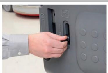
Use solution knob to adjust amount of cleaning solution being dispensed.
