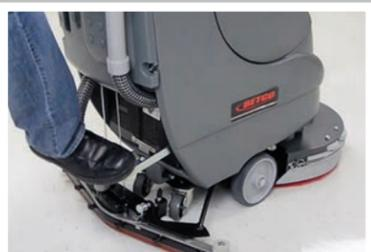
Release the pedal and place the scrub deck onto the pad driver.
