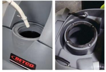
Fill machine with water and cleaning detergent. Always make sure the recovery tank is empty before each use.
