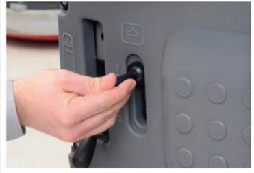
To prevent water from leaking from machine, always raise the solution knob all the way up.
