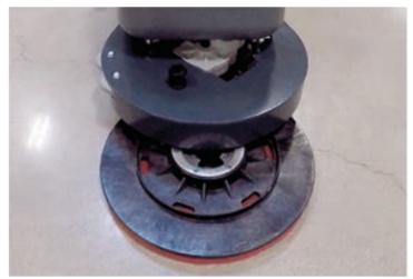
Attach clean pad to pad driver. Place pad driver on floor and center it underneath the scrub deck.
