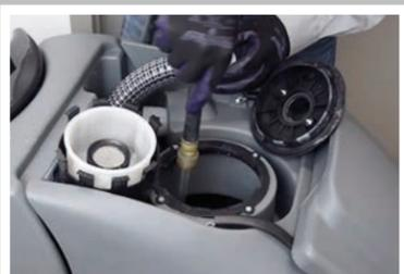
With drain hose still in mop sink, rinse recovery tank thoroughly with water. When clean and empty, attach cap and clip back onto housing.
