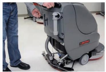
Move forward to recover any remaining water on the floor. Then, raise squeegee lever.
