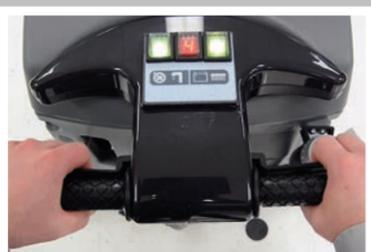
Squeeze trigger on handle to attach the pad driver.
