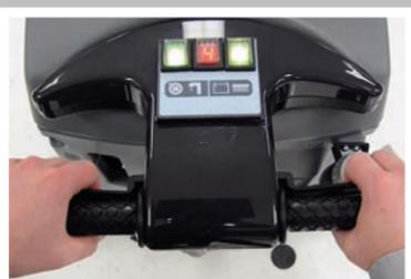
Squeeze trigger and begin moving forward to clean and dry the floor.
