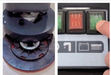
To remove the pad driver (to change or clean pad), power to the machine must be on and the pad driver still raised off the floor. Squeeze the trigger on the handle and quickly release the trigger. This will cause the pad driver to fall to the floor. Then turn off brush switch and vacuum switch.
