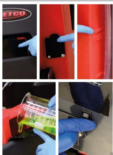
Fill the solution tank with water. If using SoliChem™ Technology, use water only in the tank. If using liquid chemical, mix chemical to recommended dilution and turn SoliChem to off.
