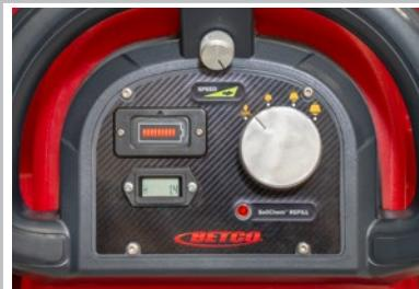
Raise scrub deck with knob by moving the knob to the head-up or transport position.
