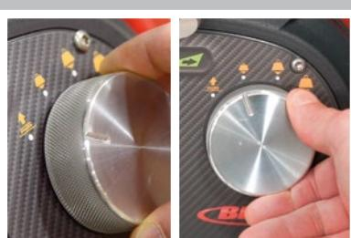
Turn key on. To attach the pad drivers, set the machine to MEDIUM (#2) down pressure setting.
