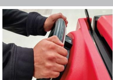
**On Disk Scrubber**, Squeeze bail on the handle to attach the pad driver. Once pad drivers are attached, adjust to desired down pressure setting.
