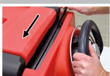
Lower the squeegee lever arm to start the vacuum to recover liquid and dry the floor.
