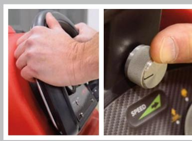
Squeeze bail on handle to move forward to clean and dry the floor. Adjust speed if necessary.
