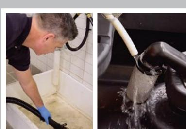
Empty recovery tank after each use. Rinse with hose while draining.
