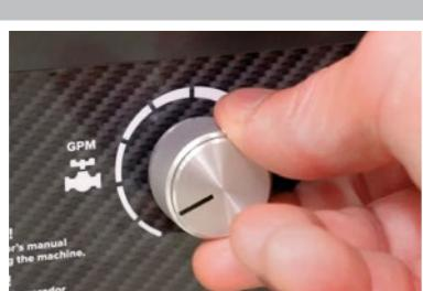
Set the cleaning solution flow rate for the cleaning application.
