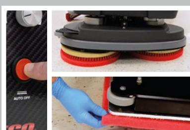
Remove the cleaning pad or pad drivers from machine. Clean or exchange as needed.
