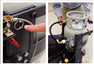
Remove the pins on the handles and move the handle to the horizontal position, then put the pins back in to lock it into position.
