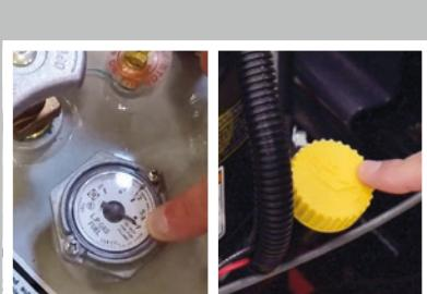
Prior to use, have the tank filled with propane and check that the engine has the proper amount of oil for operation (at the FULL line).
