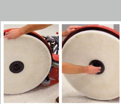
To install or replace the burnishing pad, lean the machine on its RIGHT SIDE and use the center lock to secure it in place.
