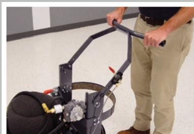
Adjust the handle to a comfortable operating position by moving the pins to the desired position. Make sure the burnishing head is on the floor when setting your desired position.
