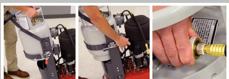
Install the filled propane tank with the tank nozzle facing forward. Then clamp it in place. Ensure the tank valve is off and finish by tightening the fuel hose to the tank valve.
