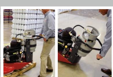
Lift slightly and rotate the rear of the machine. Once rotated so the back of the machine is perpendicular to the pallet, push down on the handle and slowly pull the machine off the pallet on the rear wheels.
