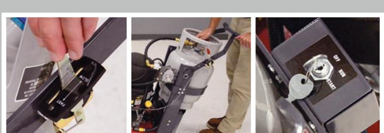
To turn the burnisher off, lift the deck off the floor and move the throttle to the slow position. Close the tank valve by turning it clockwise. The engine will stop as it runs out of fuel and then finish by turning the key to the off position.
