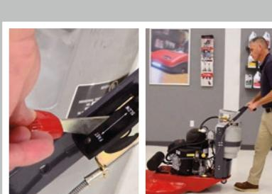
Once the machine is started, move the throttle to the FAST position. Do not operate below full throttle. Move the burnishing head down to the floor and then move forward. Do not stop without lifting the head off the ground or you can damage the finish.
