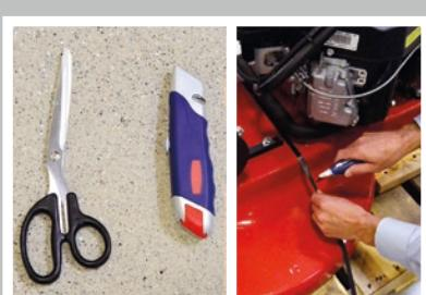
Using scissors or a razor knife, cut the banding that holds the machine to the pallet.
