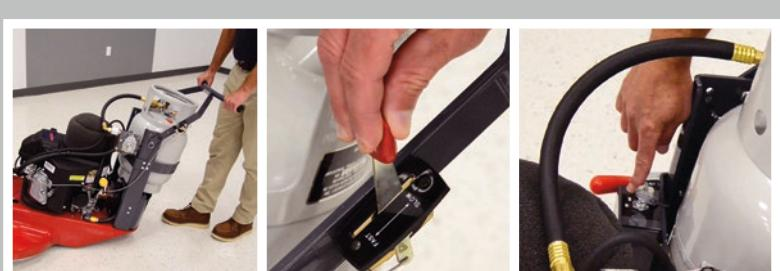
To start the machine, open the tank valve and tilt the machine back. Move the throttle to the slow position and turn the key to the start position.
